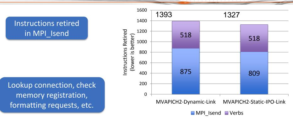
MVAPICH2-2.0rc1 (latest) code is used with default configuration options (CH3:mrail) All userspace instructions are counted for full execution of MPI\_Isend Memory copies and locks are also included in the component that uses them
