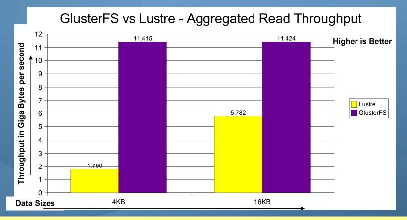
Multiple dd utility were executed simultaneously with different block sizes to read from GlusterFS filesystem.
