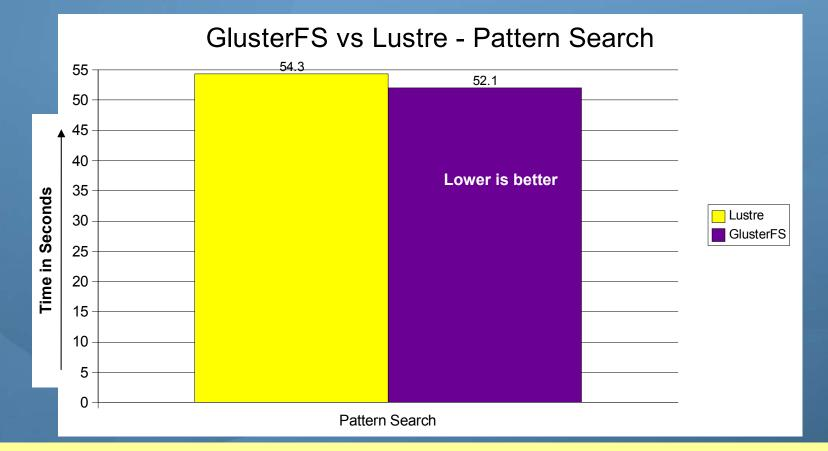
grep utility searches for a PATTERN on a file and prints the matching lines to console. This benchmark used 1GB ASCII BASE-64 file.
