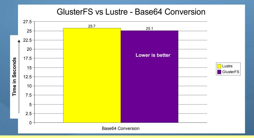
Base64 is an algorithm for encoding binary to ASCII and vice-versa. This benchmark was performed on a 640 MB binary file.
