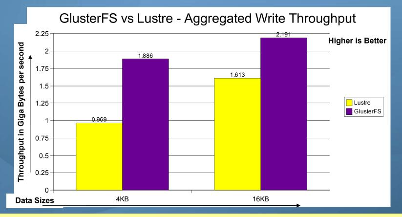
Multiple dd utility were executed simultaneously with different block sizes to write to GlusterFS Filesystem.
