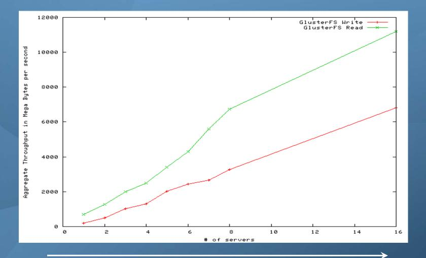
Throughput increases with corresponding increased in servers from 1 to 16
