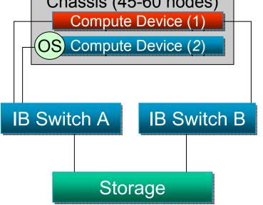
**Compute Device failure** ⇒ **Recovery is a reboot away**
